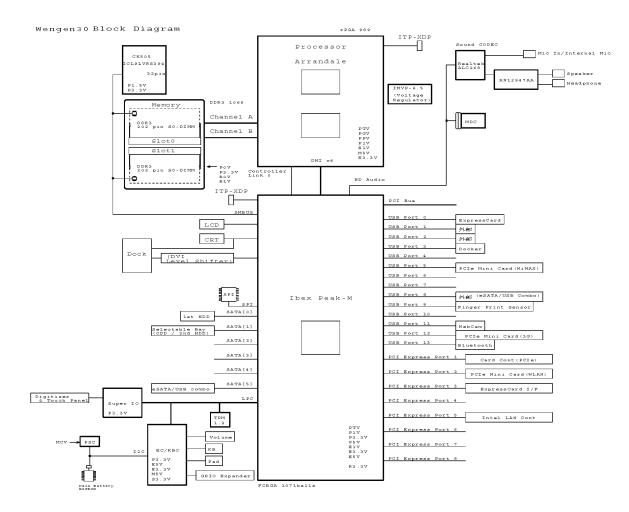
Figure 1-3 System unit block diagram
